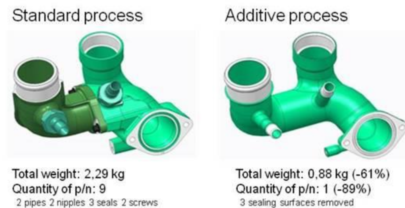
Figure 1 Design for AM resulted in subpart elimination and weight reduction
