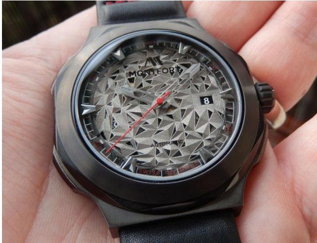
Figure 4 Monfort Strata, a crowd funded wristwatch with unusual features: a scratch-resistant, hardened steel case and a textured 3D printed dial. Made of stainless steel, the dial is made by binder jetting by Digital Metal to create a relief surface named les massifs, the motif is inspired by the Swiss Alps. With a repeating triangle pattern, the dial resembles the crystalline structure of rock, and is a visual variation of the traditional hobnail, or clous de Paris, guilloché. ( www.monfortwatches.com [27])
