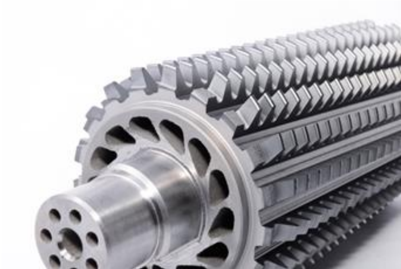
Figure 2 Milling cutter for gear manufacturing. The cutter is produced using AM in the material Vibenite®280, high alloyed HSS steel with an iron base, with a large number of carbides evenly distributed in the metallic matrix. Courtesy: VBN Components
